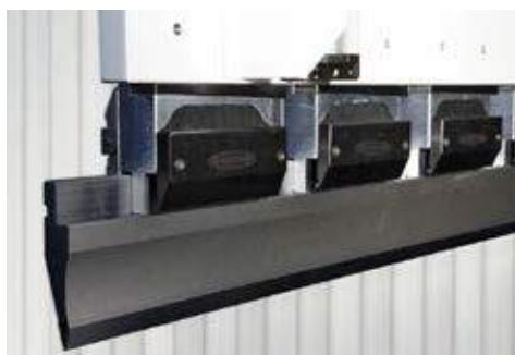
By the pneumatic clamping tools model WTC patented by Warcom, all PROMECAM tooling up to 20 Kg can be loaded from the front side. WTC moves up and block automatically the punch giving a perfect self alignment.
