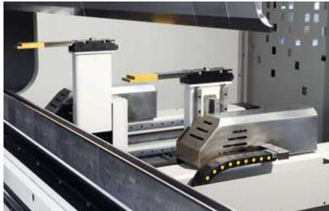
■ The new backgauge designed by Warcom is ergonomic type. The standard configuration is made with 6 axis movement managed by CNC: X1-R1-Z1; X2-R2-Z2.
